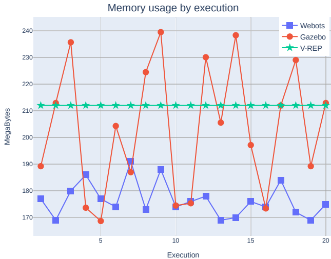
Fig. 4. The memory required for each simulator during 20 executions of the robotic scenario. The V-REP simulator presented a stable memory use (just 212MB), moreover, the Webots simulator required less memory (176.6MB average), followed by Gazebo with 203.64MB average for the task execution.
