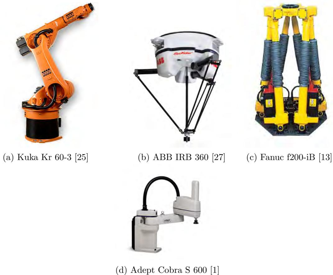
Figure 2.1: Different types of industrial robot manipulators: (a) articulated (b) delta (c) parallel/hexapod (d) SCARA
